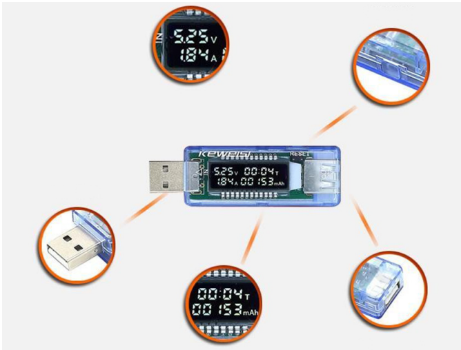
Fig. 4. Keweisi KWS-V20 USB Power Doctor and its components
